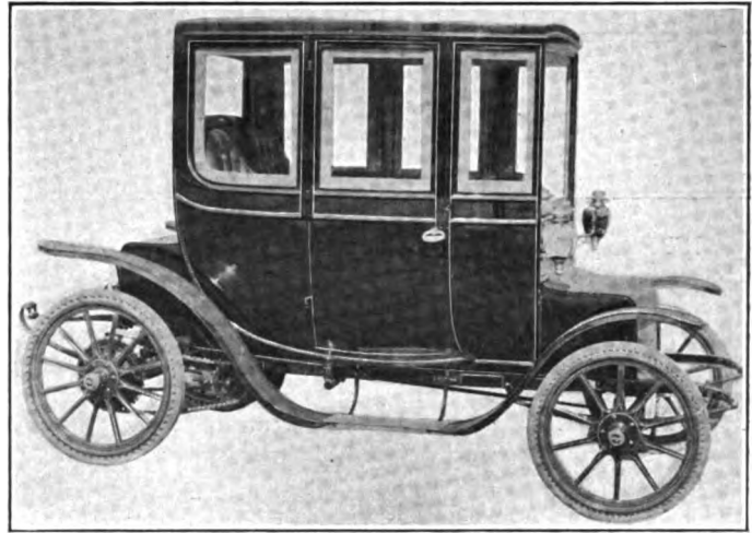
Fig. 1—Ideal Electric town car with inside control
